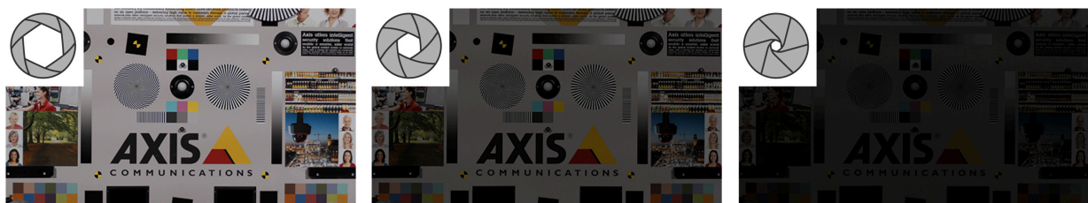
The light gathering ability of a camera is higher when the f-number is lower.
