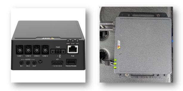
Run the coax cable for the 2 sensors through the vehcile from their install location back to the F91 main unit.
