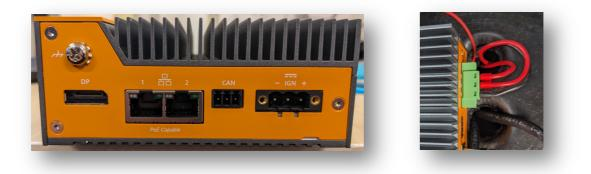
Connect the DIO terminal block to the DIO port and supply 12v dc to pin 1 and ground to pin 2.
