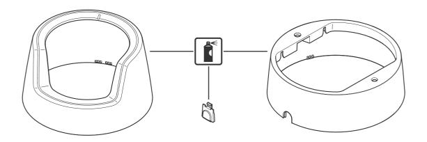
2. Apply a thin and even layer of spray paint according to the instructions of the paint manufacturer.
