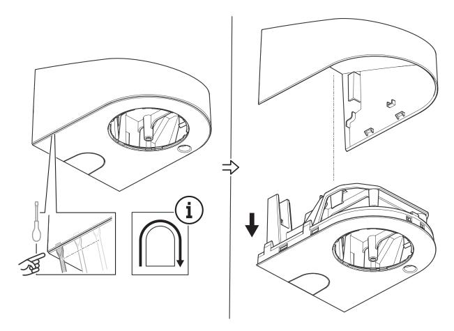
1. Use a small flathead screwdriver to loosen and remove the top cover.
