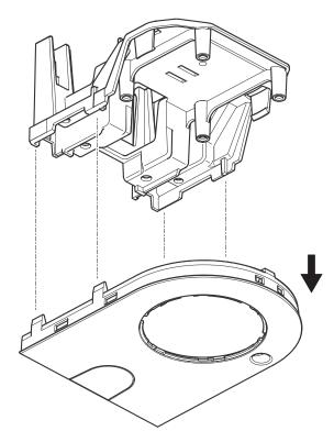
2. Gently push out the four retaining clips and remove the bottom cover.
