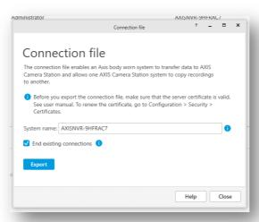
Now that the connection file has been generated, it can be applied to the in-vehicle server. Ensure that the server is connected to the same network at the central server and connect the USB drive with the connection file on it.
