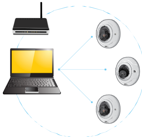
Figure 2: System set-up when client and camera located on the same network.
