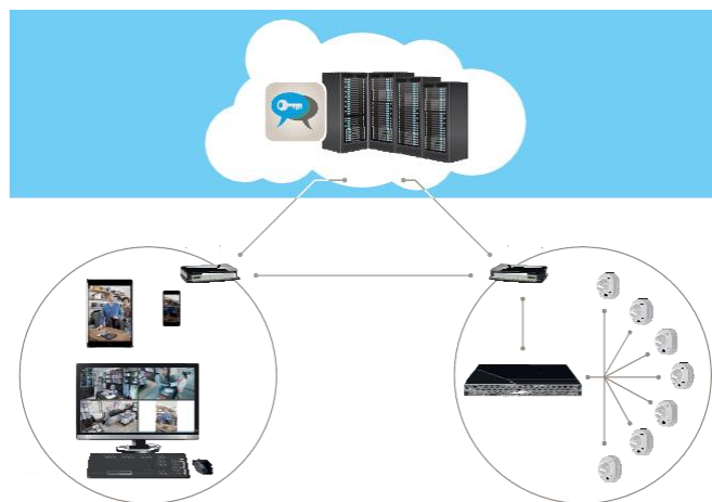
Figure 5: Secure, peer-to-peer communication between a client and a server located on different networks and fallback to relayed communication.
