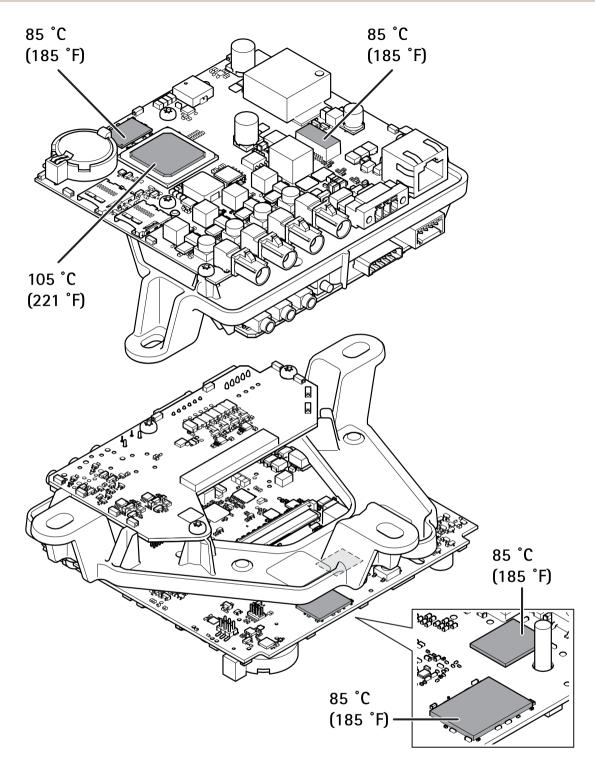
Maximum allowable temperatures. If the ambient temperature is 35  $^{\circ}$ C (95  $^{\circ}$ F) or higher, the temperature of the components increases and they must be cooled.
