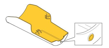
4. Mask the underside of the weathershield.
