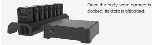
Both in-vehicle video and body worn data is offloaded to the same server.
